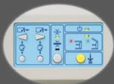
stacker unit control panel
