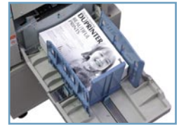
The concave receiving tray creates an air passage during the transport of documents that reduces drying time.
